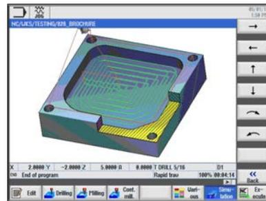
After the part is programmed it can be simulated to show the operations and tool paths. Simulation will also work with programs brought in from a CAM system that were output in G code. Cycle time is displayed also.
