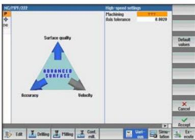
The High-Speed Machining option lets you select 3 settings for the velocity, accuracy or surface quality to produce the workpiece at extremely high speed. Includes 500 block look ahead and 1 millisecond block processing.
