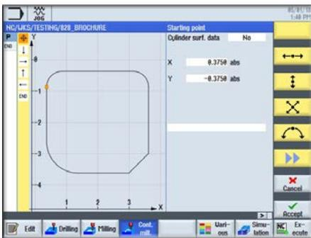
Enter part dimensions using the Simple Geometry Creator. The dimensions are drawn on the screen while you enter them and missing information is automatically calculated.
