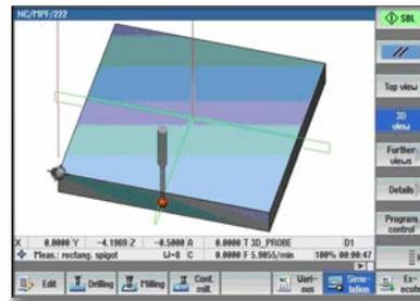
The standard part probe cycles use a simple GUI to make part set-up simple. The cycles include edge find, part skew, pocket, boss and many more. The cycles can also be used to measure the part and display dimensions on the screen, much like a CMM.
