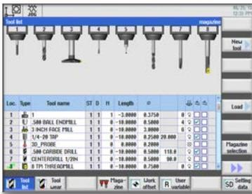
The tool management page stores your tool information in a graphical format. In addition, tools can be given tool numbers or actual names like .500 drill or .375 CBD end mill. Each tool can be managed for wear and switched automatically when the tool run time is reached.
